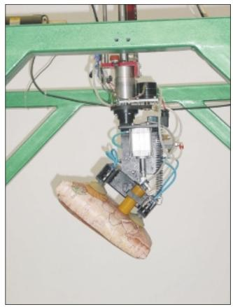
Figure 3. The gripper subsystem.
