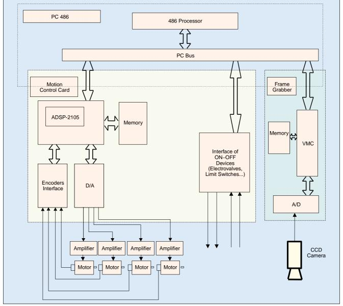
Figure 4. The overall control scheme.
