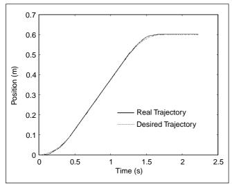
Figure 5. X-axis trajectory (displacement 0.6 m, velocity 0.5 m/s).
