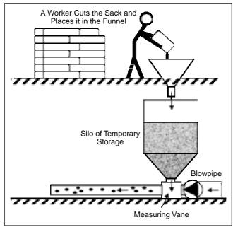
Figure 1. The depalletizing procedure.
