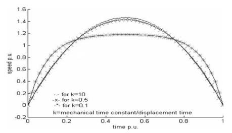
Figure 6. Optimal speed trajectories of incremental motion robot dc drives for high ( $\geqslant 0.1$ ) mechanical time constant.
