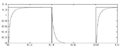
*Figure 1.* Robot dc motor speed responce as derived by the proposed control scheme "Test 1" (Speed control with simultaneous electromechanical losses minimization).
